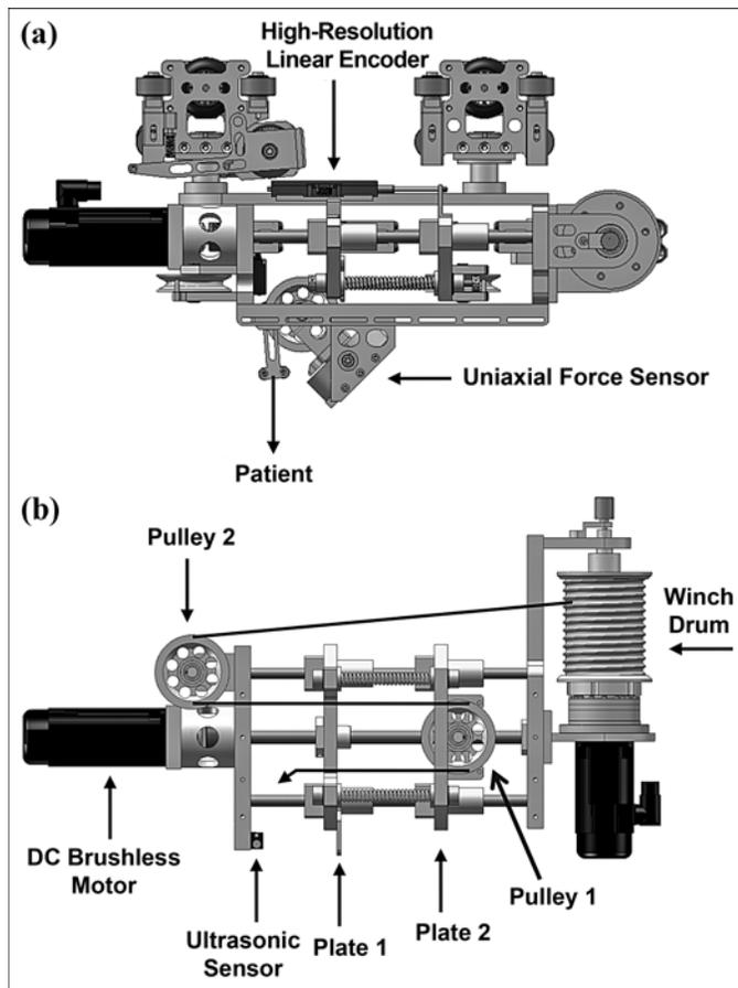
**Figure 2.** (a) Side and (b) top view of ZeroG illustrating custom-series elastic actuator that controls rope force. Note that top and bottom assemblies have been removed from (b) for clarity. DC = direct current.
